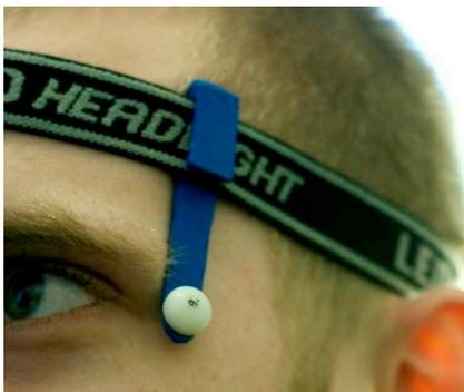
Figure 2. Eye-lens dosimeter
