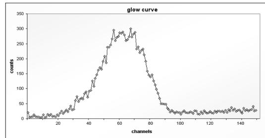
*Figure 1: Glow curve of an irradiated (at about 0.1 mSv) LiF:Mg,Ti pellet*
