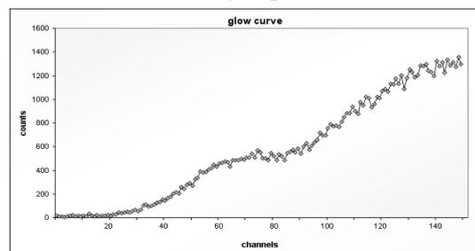
*Figure 2: Glow curve of a an irradiated LiF:Mg,Ti (at about 0.1 mSv) pellet with a high background signal at the last channels*
